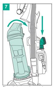
Place dust cup on base and snap into place. Store dusting brush on back of vacuum.
